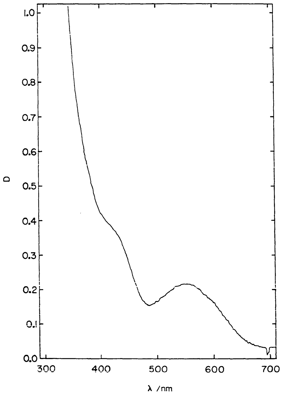
Figure I-17. The electronic spectrum of the product of the reaction of 1.4 \times 10^{-3} M Co([14]ane) ^{2+} with 1.4 \times 10^{-3} M \text{H}_2\text{O}_2
